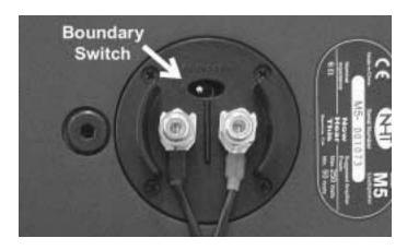
Note: The terminal plate comes from the factory oriented for horizontal placement. This allows speaker wire to hang down neatly from the speaker. The terminal plate should be rotated for vertical use. Instructions for rotating the cup can be found in section 4.2.
